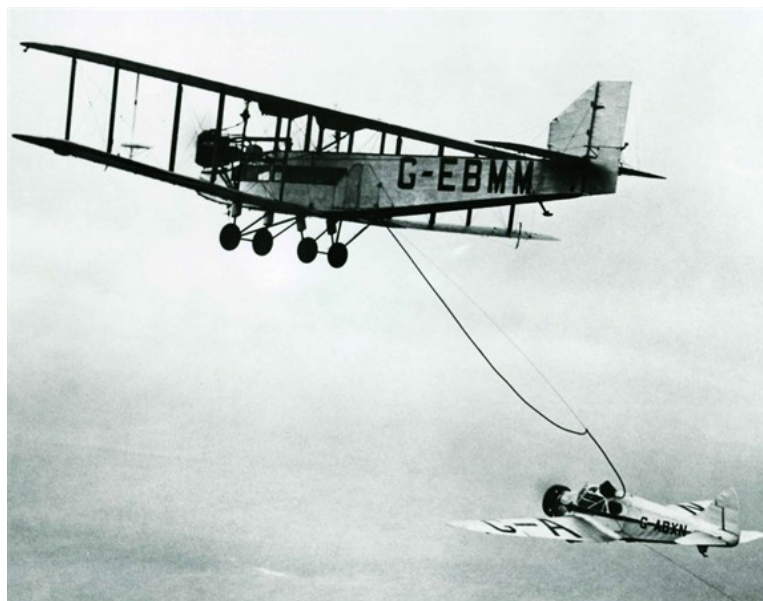
The first generation of in-flight refuelling. This picture was taken shortly after Alan Cobham's company was formed in 1934
